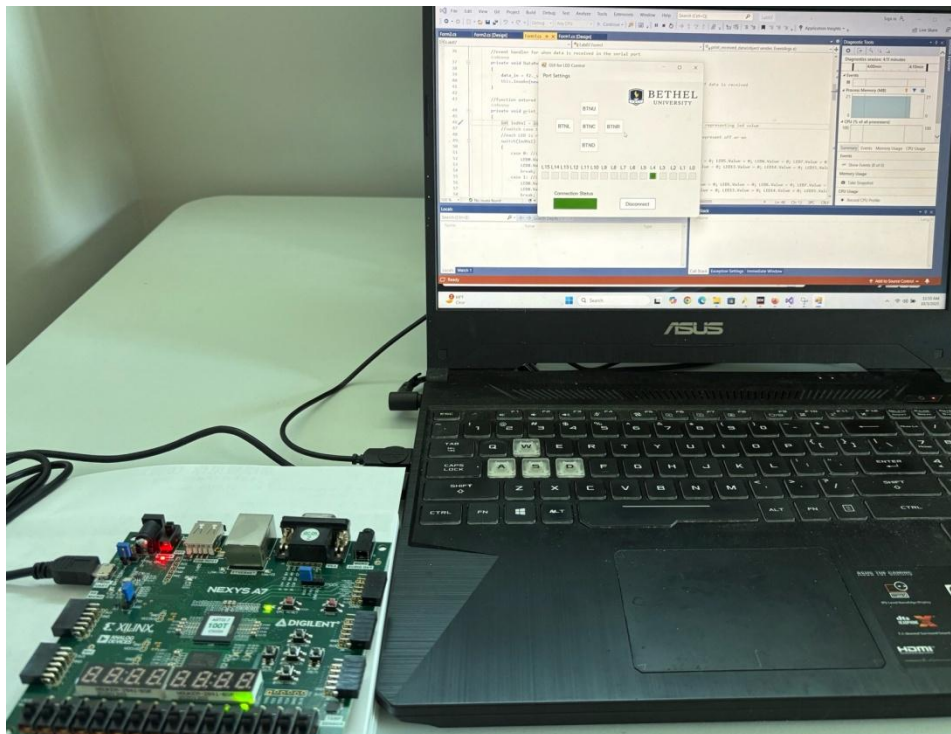
Figure 13 The regular LED operation on both FPGA board and GUI (snapshot status: Led4)
